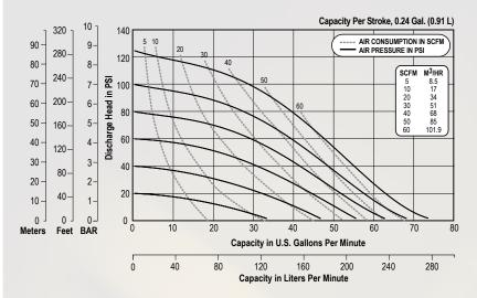
NOTE: Performance based on the following: elastomeric fitted pump, flooded suction, water at ambient conditions. The use of other materials and varying hydraulic conditions may result in deviations in excess
