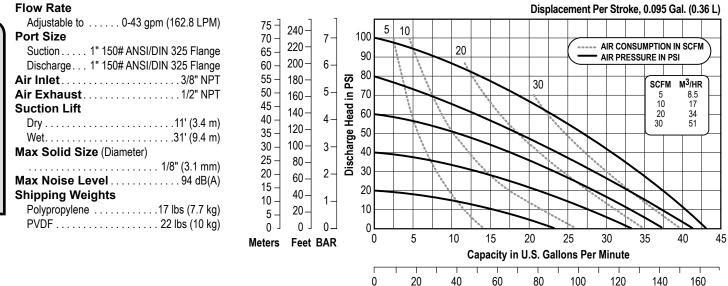
NOTE: Performance based on the following: elastomeric fitted pump, flooded suction, water at ambient conditions. The use of other materials and varying hydraulic conditions may result in deviations in excess of 5%.
